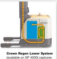
lost energy and returns it to the battery. This equates to fewer battery changes, longer shifts and reduced costs.
