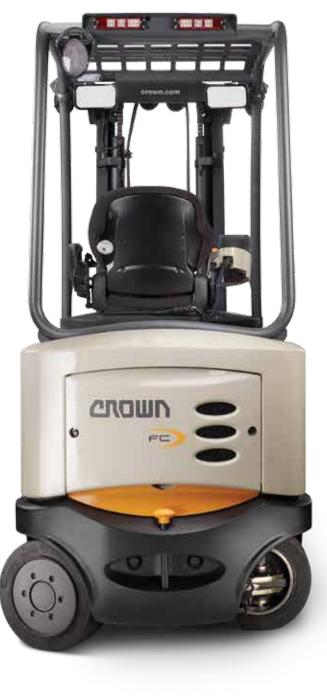
**Precise control** lets you take advantage of tighter right angle stacks. Larger, less maneuverable lift trucks require wider aisles, but drive motors turning in opposite directions allow the FC 5200 Series to spin 360 degrees in an aisle without disturbing surrounding pallets.
