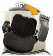
• The 15-degree pivot function, available with an optional suspension seat, gives the operator better visibility in every direction while maneuvering the truck.
