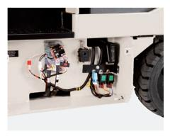
Side panel located behind left entry step offers access to relays and fuses.
