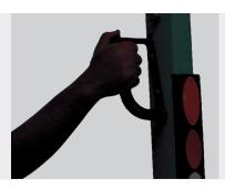
Reverse Assist Grip with Horn Provides operator control while driving in reverse. Keeps operator's hand securely inside the compartment during operation.
