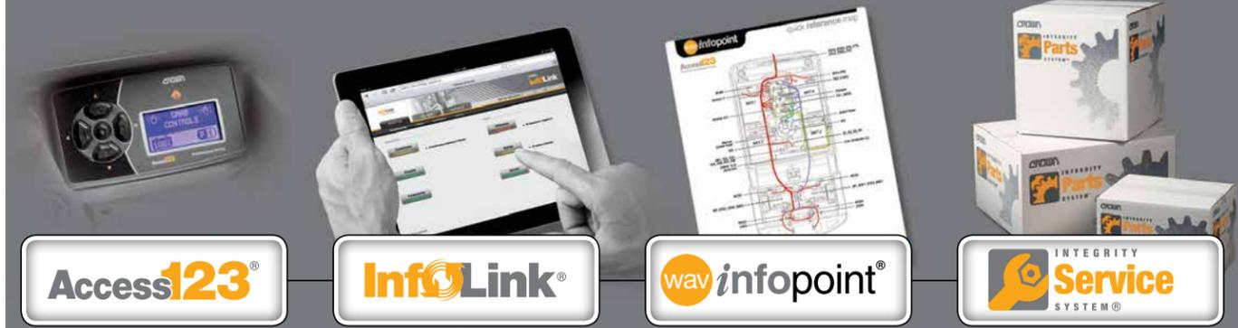
**Access 1 2 3® technology** enables advanced diagnostics through an intuitive display. This diagnostics system, used across all Crown trucks, increases technician proficiency, resulting in significant savings in service time and costs.
