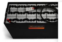
Tubular Advanced design that increases active material surface area, extending runtime for increased productivity. Bolt-on intercell connectors simplify maintenance by allowing the technician to isolate, remove and replace cells while minimizing the risk of spark or ignition. Options for high-capacity cells or standard cells with reduced watering requirements.
