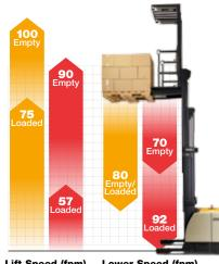
Lift Speed (fpm) Lower Speed (fpm)
