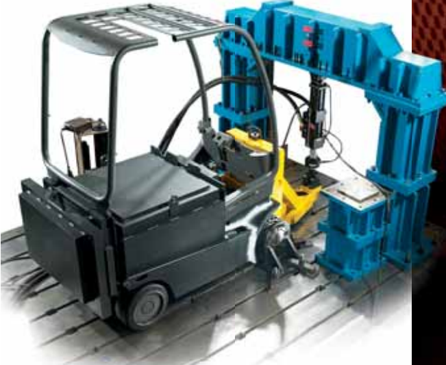
▲ Structural tests verify the frame's durability.
