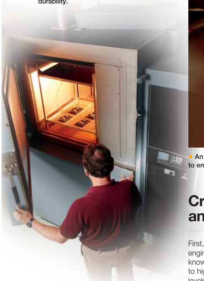
▲ Electrical components on our lift trucks are tested at -40° to 85°C to verify longevity in extreme temperatures.
