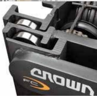
**Masts stand firm** with Crown's rigid I-beam construction, which resists longitudinal, lateral and torsional bending and twisting.
