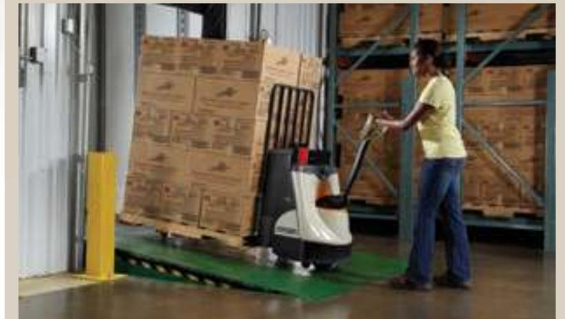
**Crown's ramp hold improves operator confidence and control** by minimizing the possibility of unexpected reverse travel when stopped on an incline. It also allows consistent speed on ramps, with or without a load.
