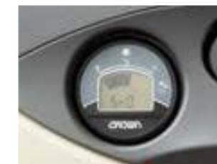
**The standard display features fault code readout** to clearly identify a system fault during truck operation or start up. No more guesswork, the display says it all.
