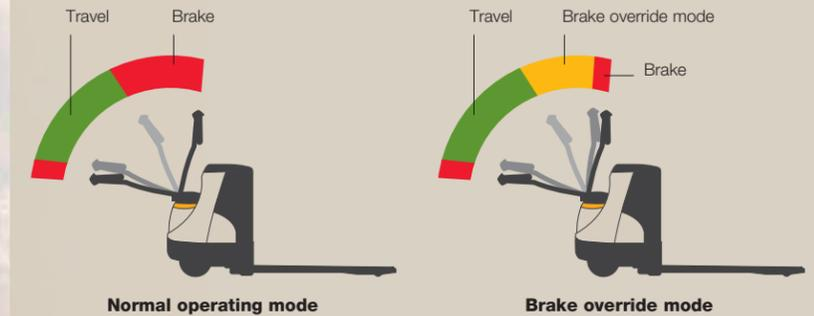
Crown gives operators the best of both worlds: in the **normal operating mode** a large brake zone ensures that operators can easily and quickly stop the truck during normal operation. When working in tight spaces, the **brake override mode** enables operators to position the handle in near vertical position while engaging traction at creep speed for fine-tuned load positioning.
