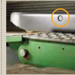
Uniquely designed to protect the forks, the riser axle on the WP 3000 Series is located at the highest point possible. This eliminates frequent repairs required when the riser axle is damaged by constant contact with dock boards, pallets and uneven floors.
