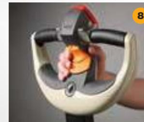
**9. Compact Design** The slim design coupled with a brake override feature allows maneuvering in tight spaces with the handle in a near vertical position while remaining within the profile of the power unit.
