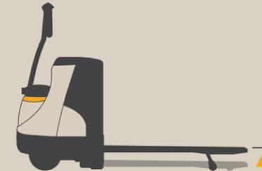
**Lift cutout at full lift** protects the motor from continuing to work once full lift is reached. This reduces energy consumption and extends component life.
