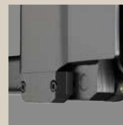
Replaceable steel wear blocks at the fork heels act as the first point of contact when underclearance is exceeded. This protects the undercarriage when driving over uneven surfaces, sharply angled dock plates or while operating on lift gates.
